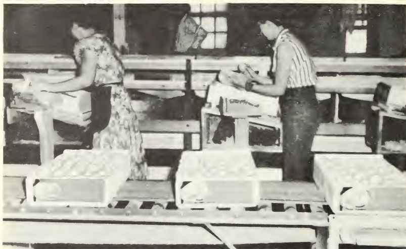
Figure 4.--Individually wrapping peaches and packing them into the standard fruit box. Packed boxes are placed on conveyor belts in foreground.
